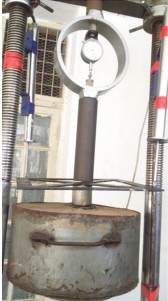
Fig. 1 Laboratory model load test on soil treated with Geopolymer column
