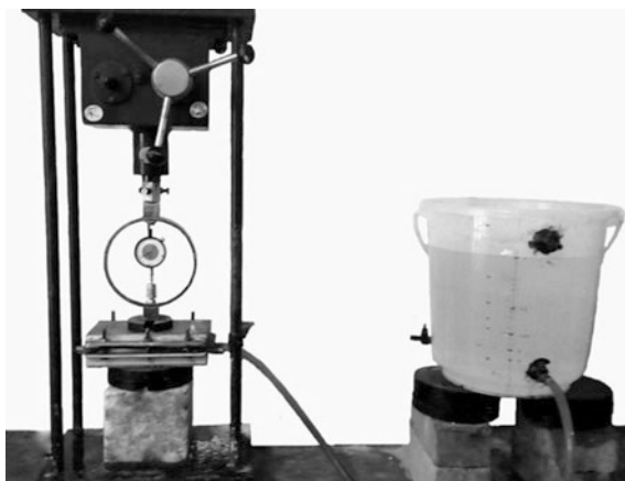
Fig. 2 Discharge capacity test set-up
