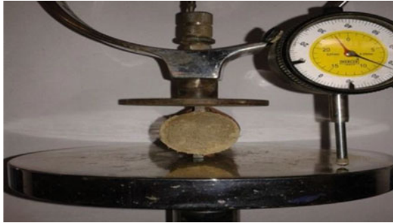
Fig. 1 Photographic view of split-tensile test
